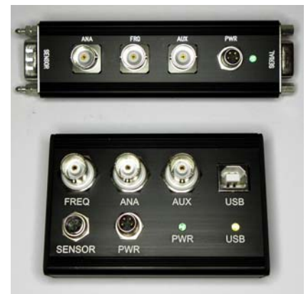
SB2 and SB3 Interconnection Box
