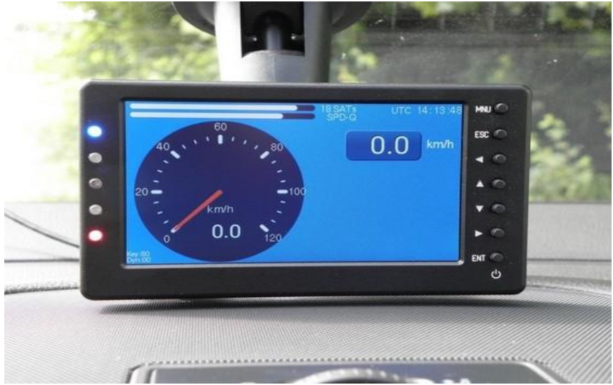
SAT200 receiver with integrated speed display, gooseneck holder and suction cup
